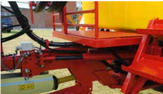
Automatic track following by means of a hydraulic drawbar with 2 cylinders.
