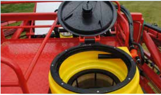
Accessible manhole with barrel cleaner for cleaning containers; easy to operate by means of corresponding pressure regulator.
