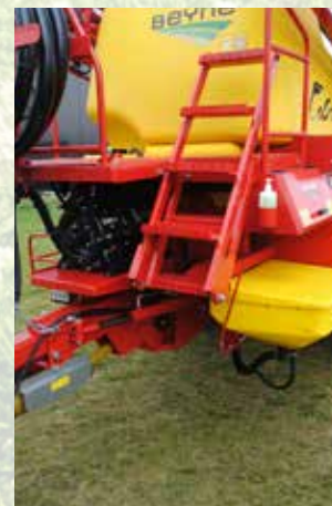
Automatic track following by means of the hydraulic drawbar, to be operated manually or via automatic zeroing.
