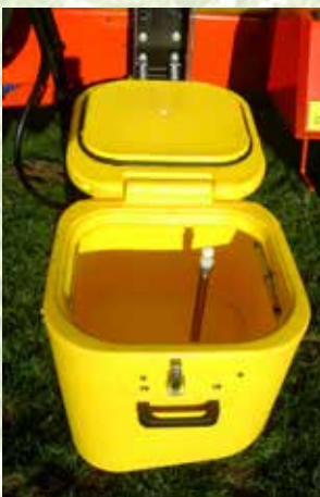
Large capacity mixing tank next to control box; also possible to easily mix in powdery chemicals.
