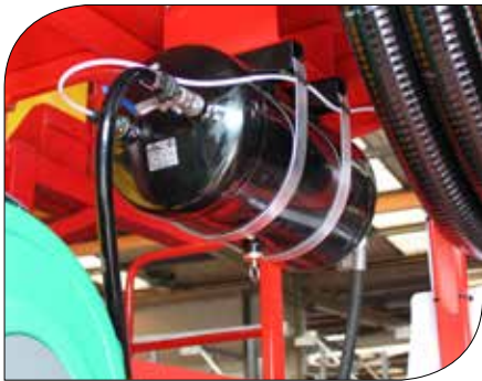
Tank with overpressure protection
