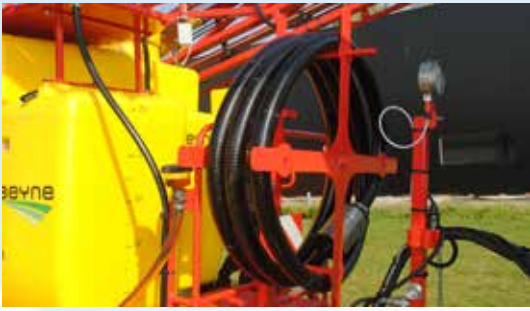
Convenient winder for storage of the suction hose (6-8 m), manually retractable.
