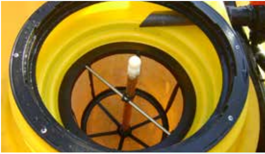
Accessible manhole with barrel cleaner for cleaning containers; easy to operate by corresponding pressure regulator.
