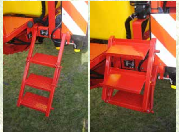
Robust stairs: easy to enter, simple to fold, takes up limited space.
