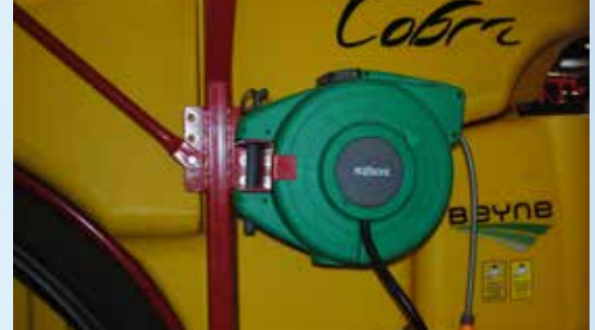
Hose reel with 20 m spray lance; to spray the machine completely clean with high pressure (10 bar).
