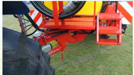
Automatic track following by means of the hydraulic drawbar, to be operated manually or via automatic zeroing.
