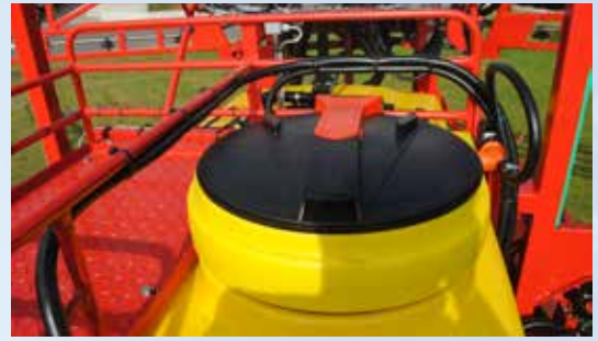
Manhole with easily accessible platform for storing chemicals.
