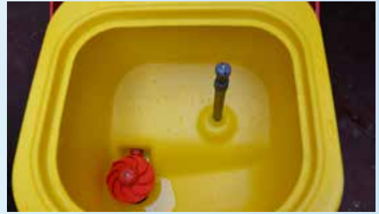
Large capacity mixing tank adjacent to the panel; also possible to easily mix in chemical powders.
