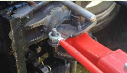
Easy to set control of steering via the adjustable handle bar (fully mechanical transmission).
